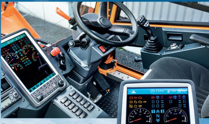
The operating concept, implemented according to the most recent knowledge, consisting of a coloured display, a multifunctional control knob and a joystick.
