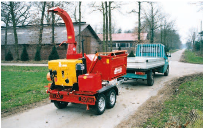
Wood chipper HM 250, mounted on one-axle chassis with turn ring
