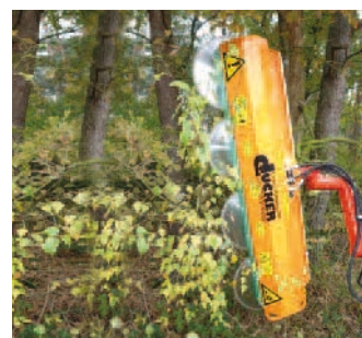
LPS 20 Clearance-Gauge-Cutter Working width: 2000 mm Revolutions of saw blades: 2600 rpm Weight: approx. 220 kg
