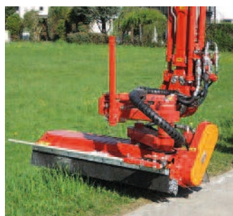
TTM 13 Flail-Mower-Head Working width: 1300 mm Revolutions of shaft: 2800 rpm Weight: 270 kg
