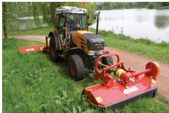
UMT as fine cutting flail-mower
