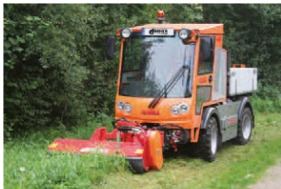
UMT 15 with hydraulic drive, front mounting
