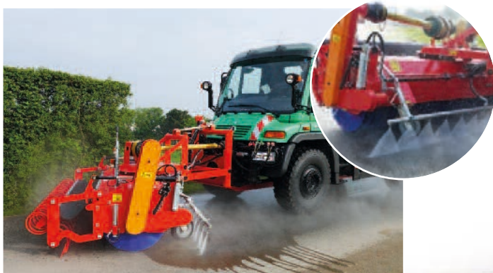
SFK with dirt scratch-ledge and water high-pressure spraying unit
